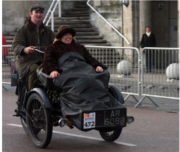
1904 Lagonda Forecar, Twin-cylinder, 12 h.p
